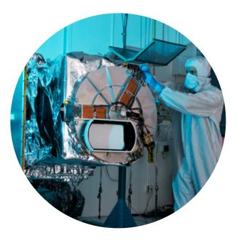
Ball Aerospace built the Tropospheric Emissions: Monitoring of Pollution (TEMPO) instrument for NASA. Once launched, TEMPO will measure and observe air pollution hourly during daytime over North America
