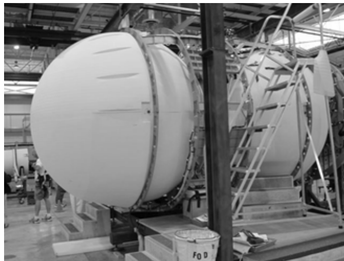
Figure 6. Completed, insulated tanks installed into Phantom Eye airframe.
