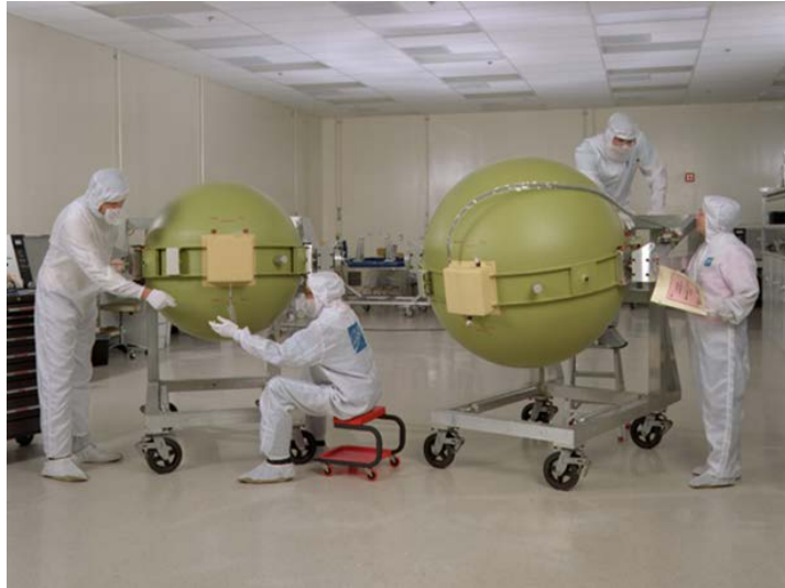
Figure 4. PRSA Oxygen and hydrogen tanks in tooling fixtures
