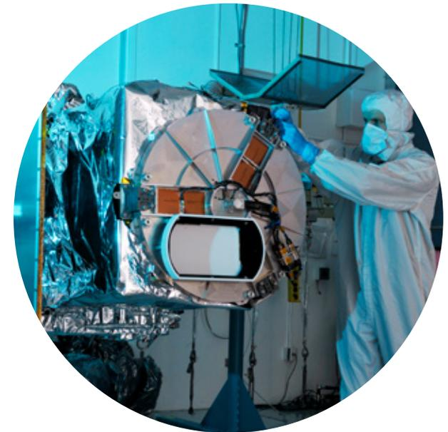
Ball Aerospace built the Tropospheric Emissions: Monitoring of Pollution (TEMPO) instrument for NASA. Once launched, TEMPO will measure and observe air pollution hourly during daytime over North America
