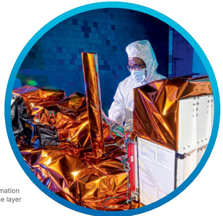
The Ozone Mapping and Profiler Suite instruments, built by Ball Aerospace, provide critical information on the health of the Earth's ozone layer
