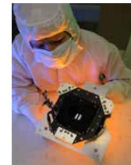
The Cloud, Aerosol, Water Vapor, Ice, Snow (CAVIS) atmospheric instrument aboard the commercial imagery satellite, WorldView-3, also built by Ball, provides atmosphere correction data to improve WorldView-3's imagery. Ball was able to provide the CAVIS instrument at a fixed-price and substantial cost savings by using a modular and command product for the electronics designs, focal plane detectors and spectral filter.
