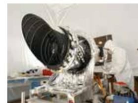
Ball designed and built the High Resolution Imaging Science Experiment (HiRISE), a high-resolution camera, for NASA's Mars Reconnaissance Orbiter mission. HiRISE is the largest telescopic camera ever sent into orbit around another planet and is able to identify images as small as a coffee table.
