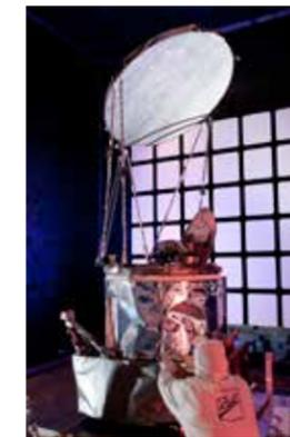
This Ball-instrument is setting the new standard for calibration for the scientific community's radiometer needs. This imager is central to the Global Precipitation Measurement (GPM) mission's success by allowing for temporal sampling of rainfall accumulations, as well as more frequent and higher quality data collection.
