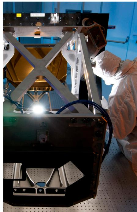
*Ball technician inspects the Webb telescope Aft Optics Subsystem during mirror integration activities*
